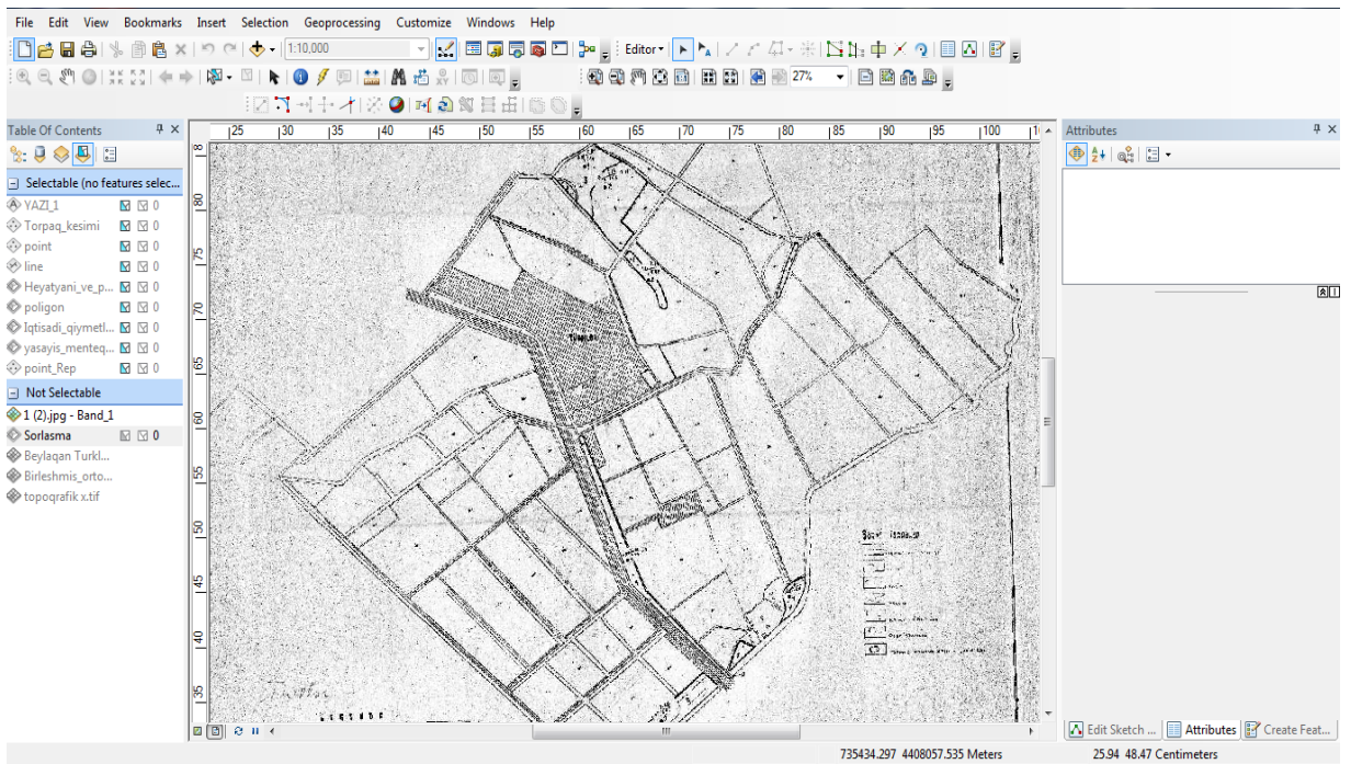
Fig. 2. Connecting view of the salinisation map of the soils of Turkler village with the coordinate in ArcGIS
