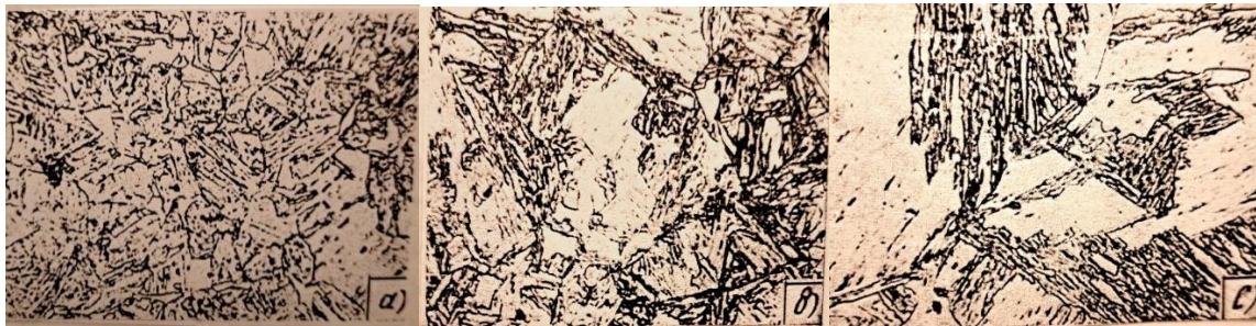
Figure 6. Microstructure of pashtos cured at different temperatures (x500)
