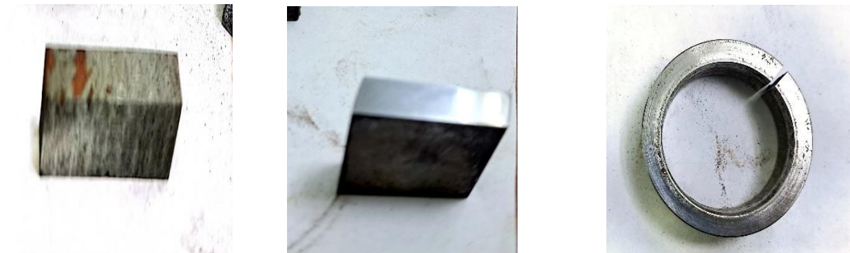
Figure 1. Macro view of samples cut from pistah a) 10 \times 10 \times 55 b) 20 \times 20 \times 100 c) pipe section
