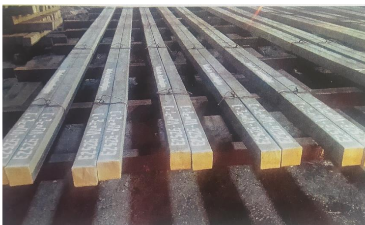
Figure 7. General view of 125 \times 125 mm square pistahs.
