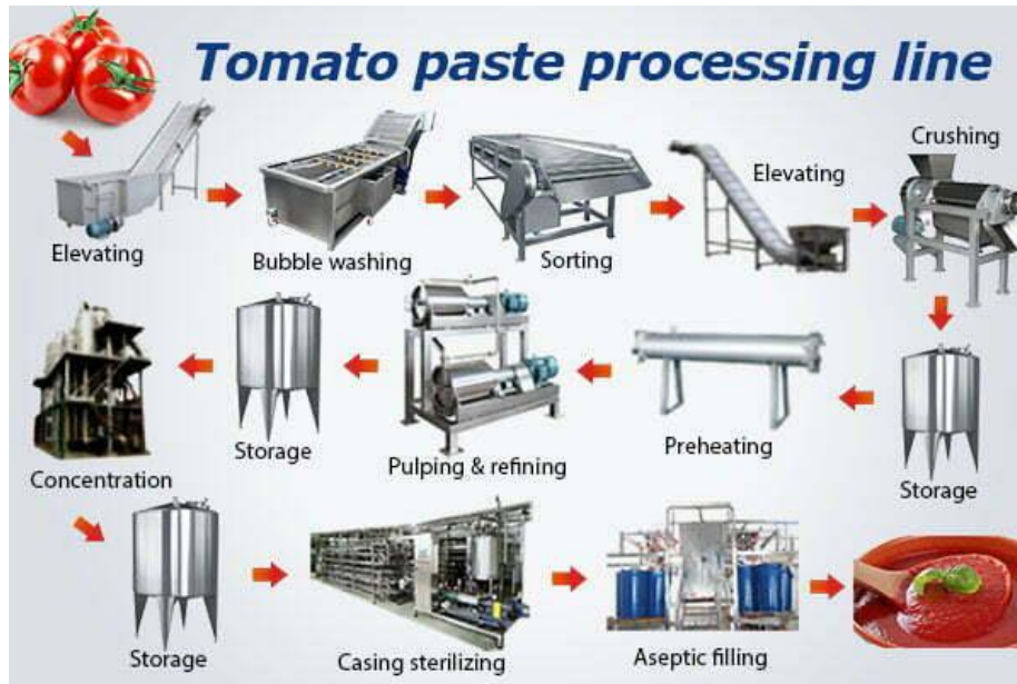
Figure 1: Tomato paste processing line
