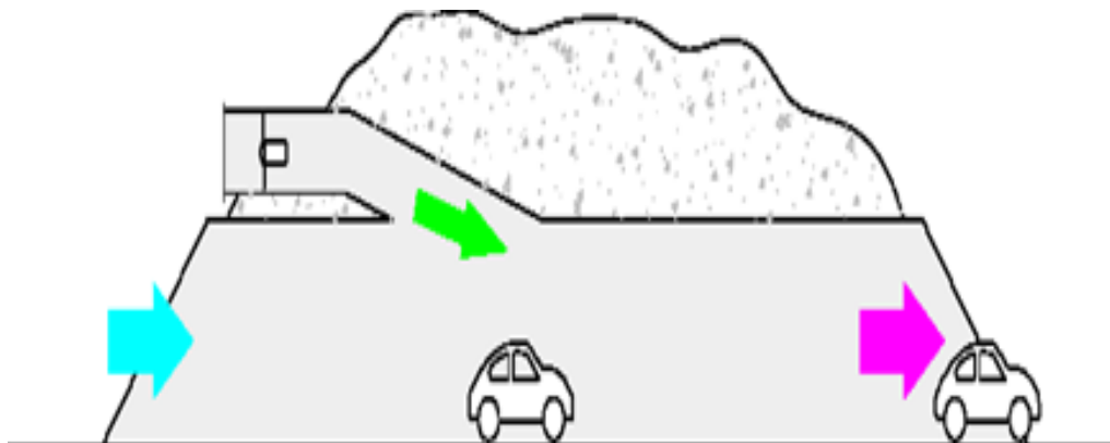
Figure 1. Sakardo heads allow outside air to enter through fans located in a fan chamber at the edge of the tunnel
