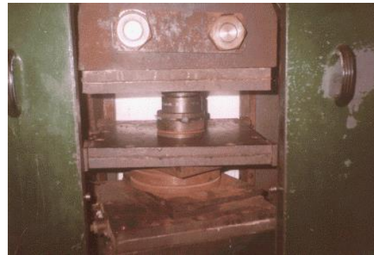
Fig. 1. Pressing the material filled in the press mold in a hydraulic press
