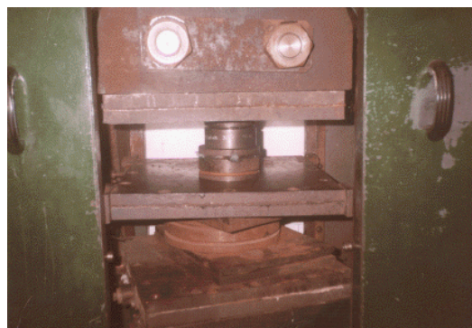
Fig. 1. Pressing the material filled in the press mold in a hydraulic press
